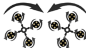
SISTEMA PLANETARIO CONTROROTANTE Planetary counter-rotating system
